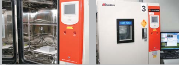
Thermal testing is performed on the WEBS system inside the calibrated chamber with defined temperature conditions
